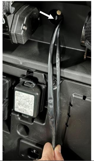
**Step 9:** Pull the connectors from the rear side of the firewall. Route the light bar connectors up the chassis member where the RTL is mounted. Connect the RTL leads to the mounted light bar by matching color to color.
