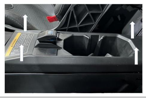
**Step 16:** Carefully pull out the switch panel on the lower console. This will create an empty space that would be used to pull the spade connectors for mounting the switches.
