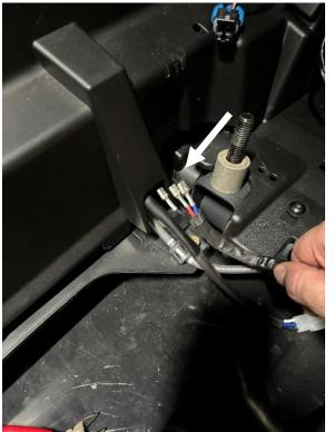
**Step 18:** Use the photos taken of the backlight switch pin outs and connect the switches.
