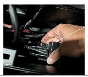
Tie the Turn signal relay to the harness using zip ties inside the lower console compartment.
