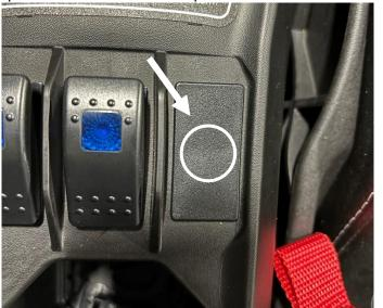
**Step 19:** Push the switches inside the panels so they are locked in their place.
